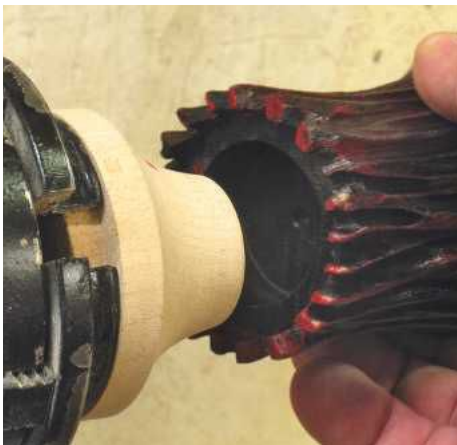
▲ Pic.16 When the red is dry give the whole thing a couple of coats of gloss lacquer. Les turned a plug for the hole in the end to act as a friction drive and allow him to turn away the spigot
